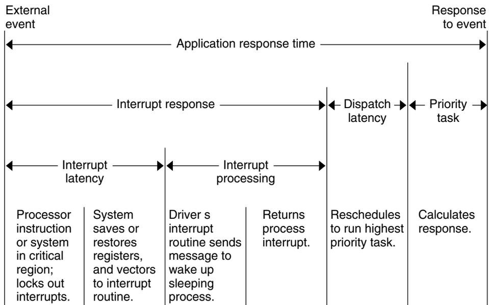
The overall application response time consists of the interrupt response time, the dispatch latency, and the application's response time.
