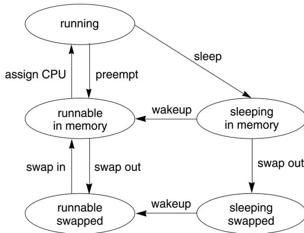
An active process is normally in one of the five states in the diagram. The arrows show how the process changes states.
