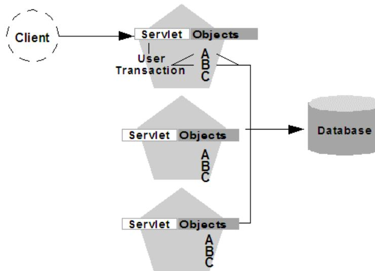
In this example, a client attaches to the first WebLogic Server instance in the cluster and obtains a `UserTransaction` object. After beginning a new transaction, the client looks up Objects A and B to do the work of the transaction. In this situation WebLogic Server always attempts to use replicas of A and B that reside on the same server as the `UserTransaction` object, regardless of the load balancing strategies in the stubs for A and B.
