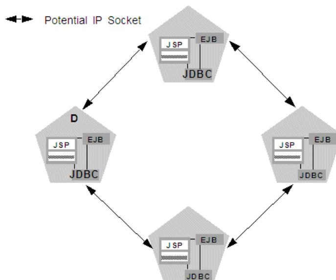
The two sockets in this example are used to replicate HTTP session states between primary and secondary server instances. Sockets are not required for accessing clustered objects, due to the collocation optimizations that WebLogic Server uses to access those objects. (These optimizations are described in [Section 5.2.6, "Optimization for Collocated Objects."](#)) In this configuration, the default socket reader thread configuration is sufficient.
