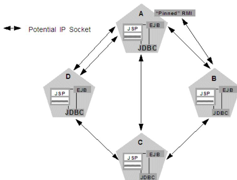
In this example, each server instance can potentially open a maximum of three sockets at a given time, to accommodate HTTP session state replication and to access the pinned RMI object on Server A.
