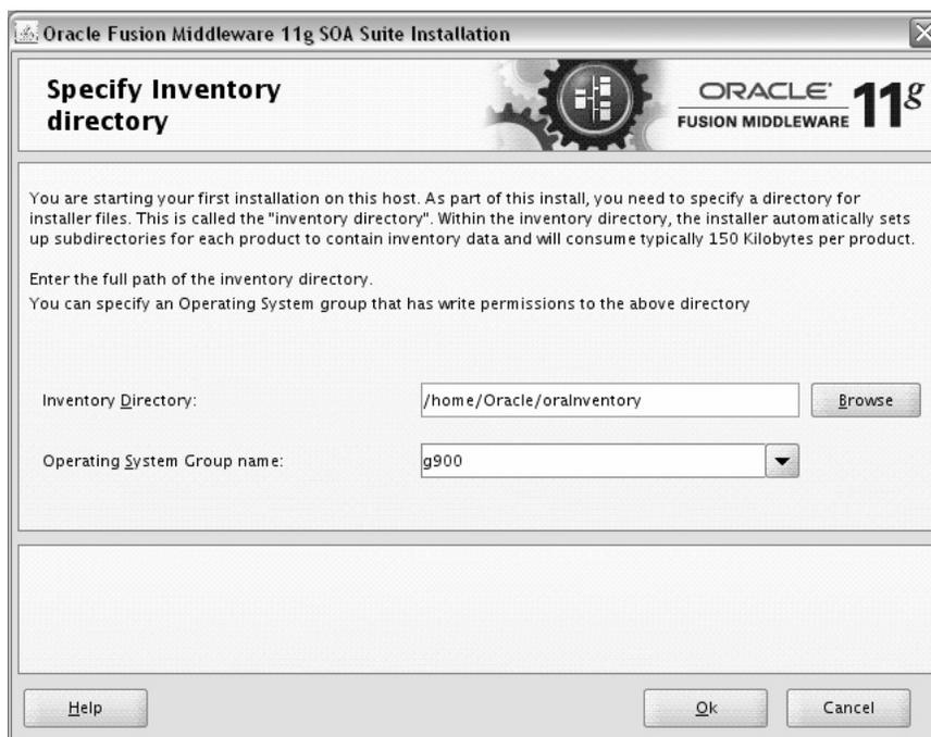
This screen appears for UNIX systems only; if this is your first Oracle installation on this host, you must specify the location of the inventory directory. This inventory directory is used by the installer to keep track of all Oracle products installed on the computer.
