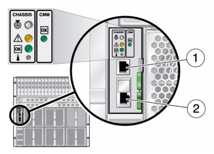
The following illustration shows the CMM that is supported with the A90-D and 7105379 chassis. The CMMs for these chassis have different part numbers, but they have the same layout.
