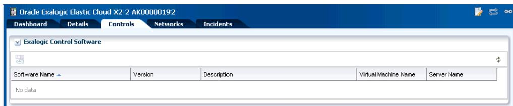
You can select any Exalogic Control component in the table and double-click to view the dashboard for each component. This table helps you identify where the Exalogic Control software components are running in your Exalogic machine. Use the **Refresh** icon on the Exalogic Control Software pane to refresh the list, when needed.
