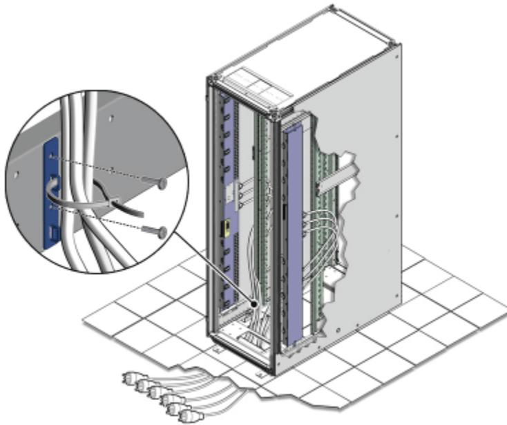
**Figure 3-10 Power Cord Routing Example from the Top of the Rack**
