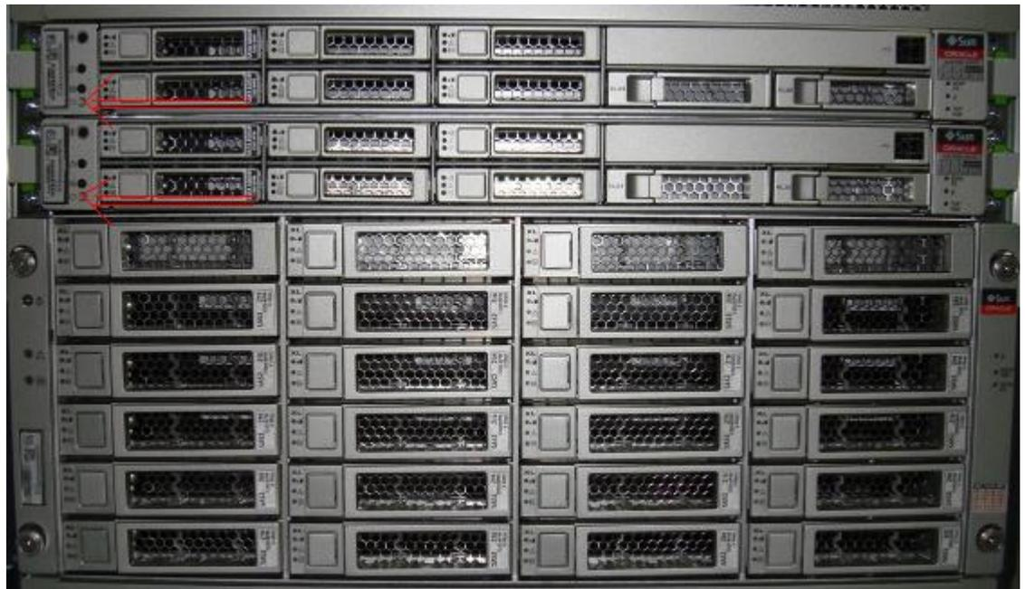
Figure 3-14 shows the soft switch and LED lights on each of the server heads in the storage appliance.
