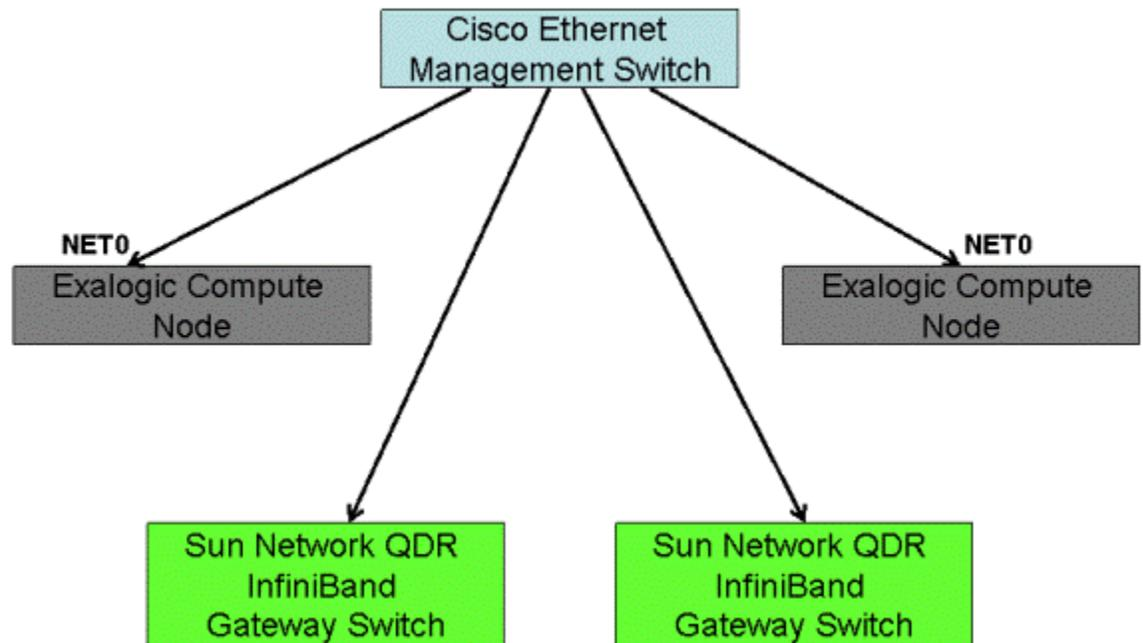
Figure 7-1 shows two compute nodes and two Sun Network QDR InfiniBand Gateway Switches as an example only. The number of compute nodes and gateway switches depends on your purchased Exalogic machine rack configuration. The Cisco Ethernet management switch is connected to the `NETO` port of compute nodes, and it is connected to the InfiniBand gateway switches.
