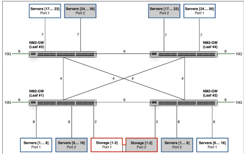
In Figure C-4, **NM2-GW** represents a Sun Network QDR InfiniBand Gateway Switch (leaf switches). **Servers** refers to compute nodes in the Exalogic machine.
