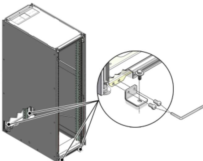
5. Using bolts and washers that are appropriate for your installation site, permanently mount your system to the floor using the four mounting brackets as shown in [Figure 3-7](#).
