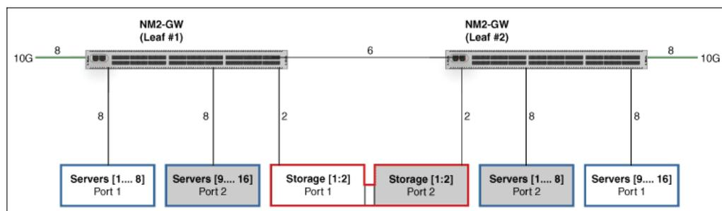
In Figure C-3, **NM2-GW** represents a Sun Network QDR InfiniBand Gateway Switch (leaf switches). **Servers** refers to compute nodes in the Exalogic machine.
