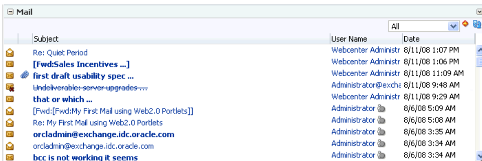
Figure 36–9 A Mail Task Flow where the Region Parameter Tabular Is Set to True
