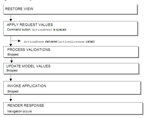
Figure 5–3 Lifecycle for Command Button Set to Immediate
