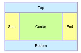
Figure 9–9 Facets in the panelStretchLayout Component
