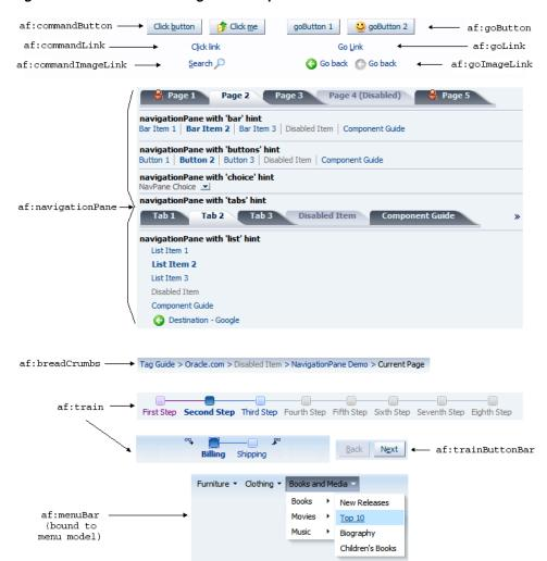
Figure 20-1 ADF Faces Navigation Components
