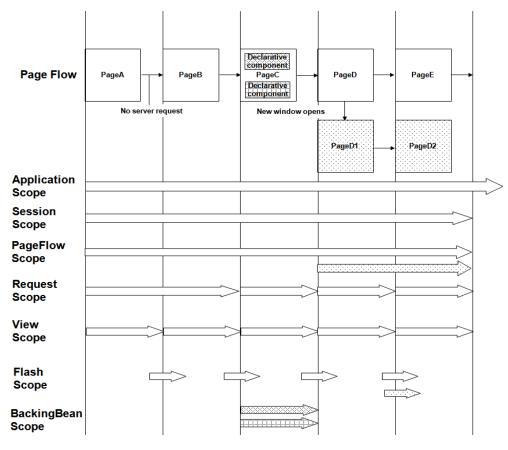
Figure 5-11 Relationship Between Scopes and Page Flow
