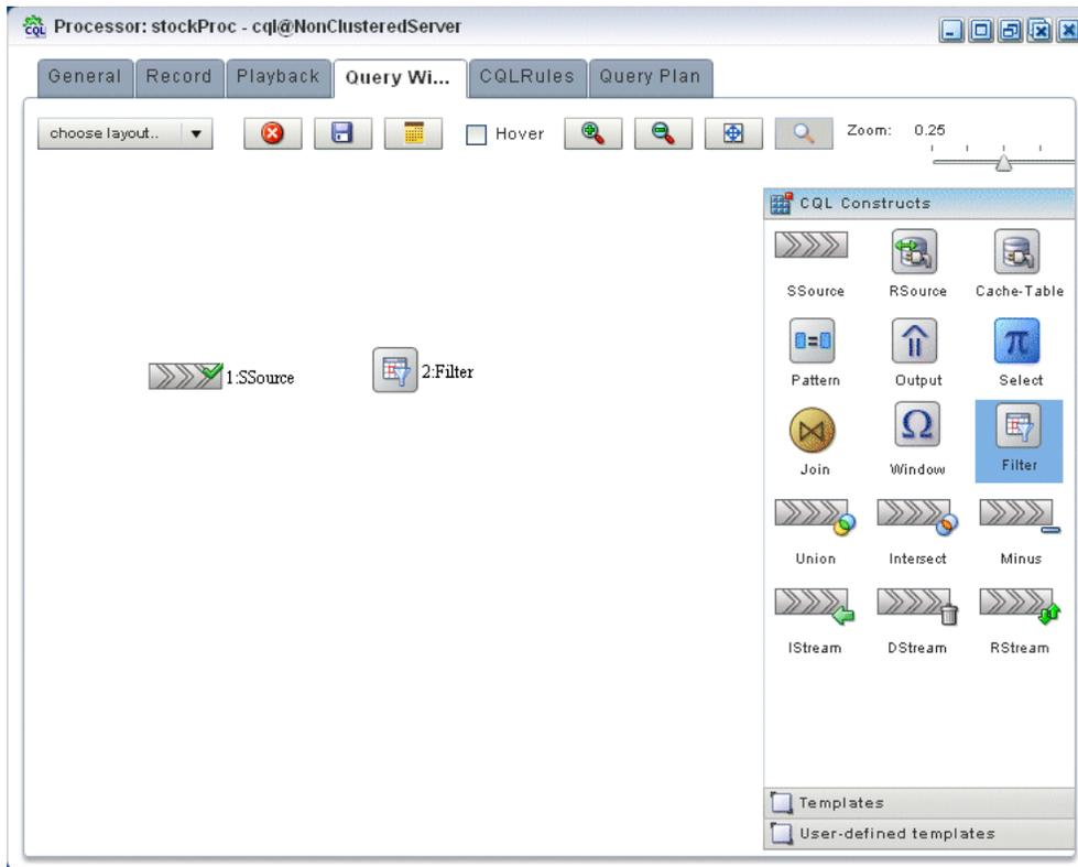
15. Click on the SSource icon and drag to the Window icon to connect the Oracle CQL constructs as [Figure 3–48](#) shows.
