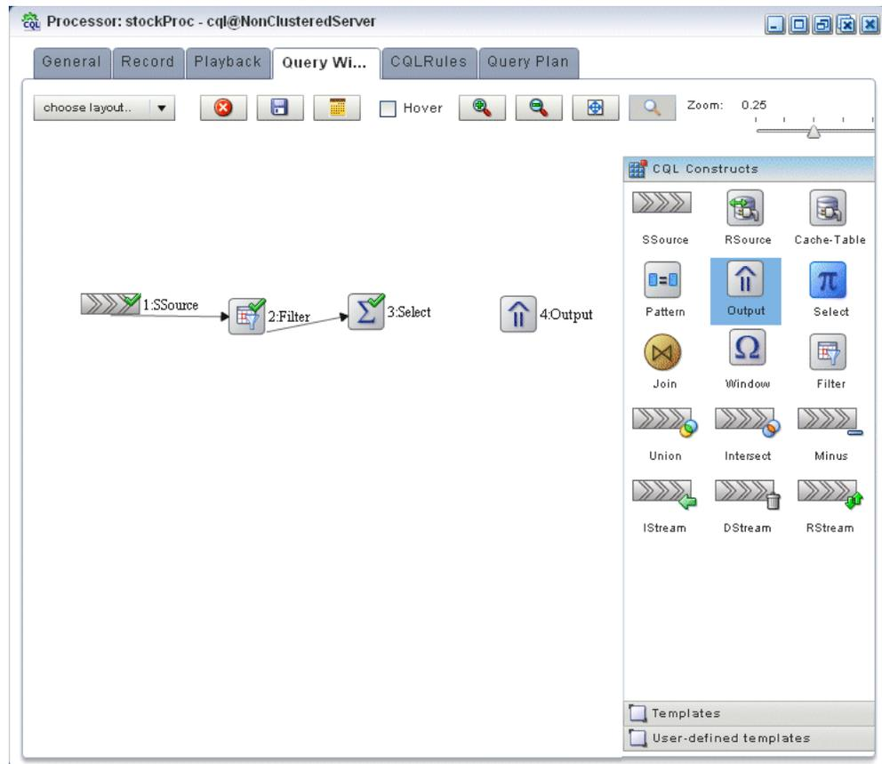
30. Click on the **Select** icon and drag to the **Output** icon to connect the Oracle CQL constructs.
