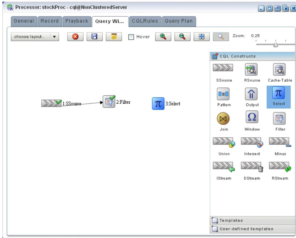
24. Click on the **Filter** icon and drag to the **Select** icon to connect the Oracle CQL constructs.
