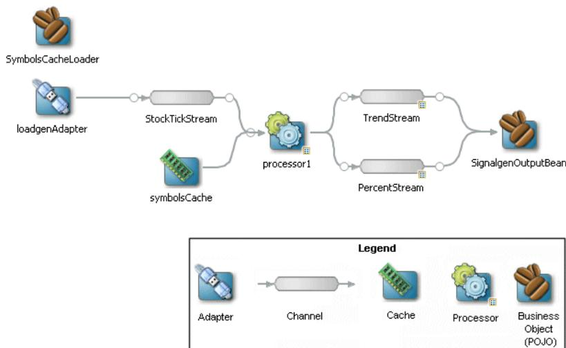
The application simulates a market data feed using the Oracle CEP load generator utility; in this example, the load generator generates up to 10,000 messages per second. The example includes an HTML dashboard which displays the matched events along with the latencies; events consist of a stock symbol, a timestamp, and the price.
