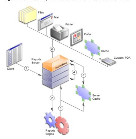
Figure 13–1 Main components of destination/distribution architecture
