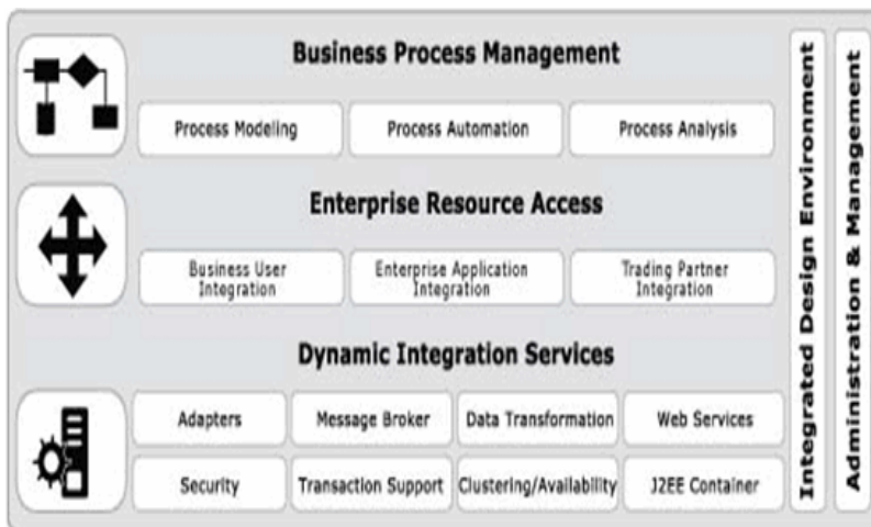
Figure 1-2 Functional Overview of WLI
