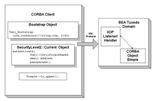
Figure 3-6 How Certificate Authentication Works
