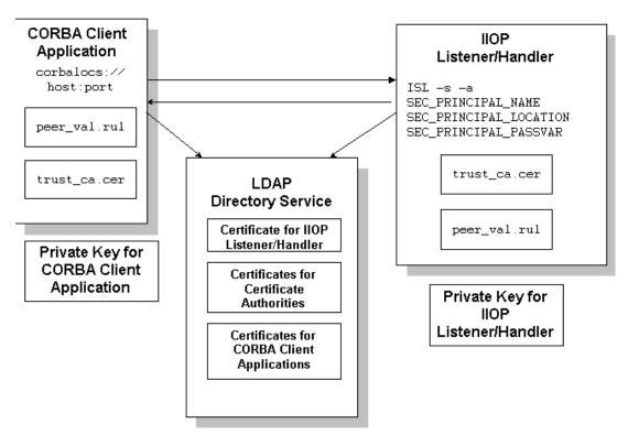
Figure 3-7 Configuration for Using Certificate Authentication in a CORBA Application
