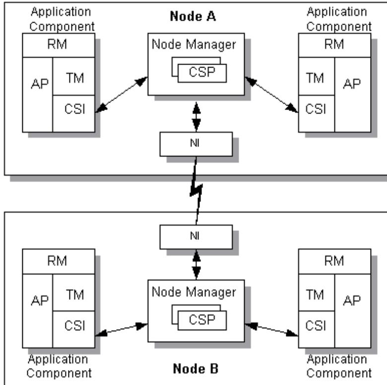
As shown in the figure, a BEA TOP END system consists of one or more nodes. A basic node consists of a client, a node manager, and a server.
