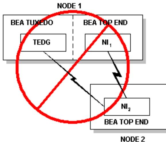
As you can see in the diagram, a single physical node, NODE 1, can support two logical nodes: the TEDG on the BEA Tuxedo system and NI<sub>1</sub> on the BEA TOP END system. In this scenario, the TEDG on NODE 1 is capable of functioning as an NI to NI<sub>2</sub> on NODE 2. The TEDG cannot be used to connect to NI<sub>2</sub> on NODE2, however, if another NI (in this case NI<sub>1</sub> on the BEA TOP END system on NODE 1) is connected to that node.
