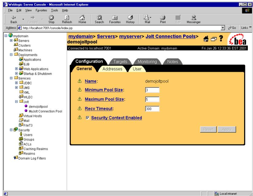
For each Jolt connection pool there is an individual MBean that displays the pool name, maximum connections, pool state, and statistics about the connection status.
