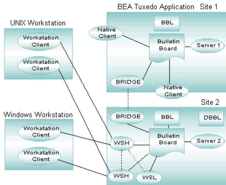
Two workstation clients are running on a UNIX system; another two Workstation clients, on Windows 2000. All workstation clients initially joined the application through the Workstation listener (WSL), which delegates subsequent communication to a Workstation handler. This process differs from the process that occurs when native clients join an application: in the latter case, the native clients attach directly to the bulletin board upon joining.
