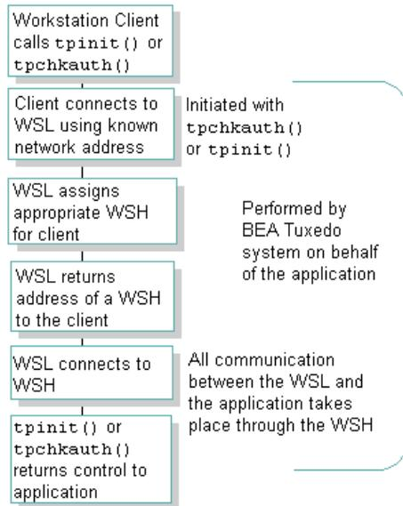
The client connects to the WSL process using a known network address. The process for establishing this connection is initiated when the client calls `tpchkauth()` or `tpinit()`. The WSL returns the address of a WSH to the client, and then notifies the Workstation handler process of the connection request. The WSC connects to the WSH. All further communication between the WSC and the application takes place through the WSH.
