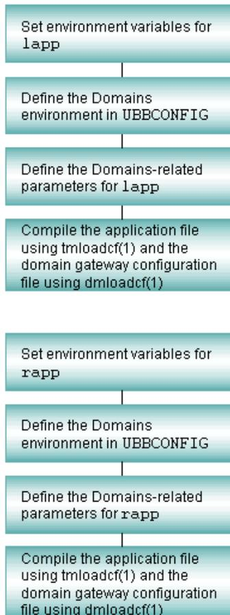
The following diagram shows which sections of the `UBBCONFIG` and `DMCONFIG` files you need to configure for a two-domain application. One domain represents the local domain; the other, the remote domain.
