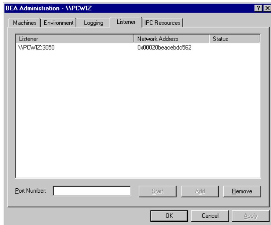
During the BEA Tuxedo installation, the installer program installed a Tlisten service on your Windows Server 2003 system. Each time you boot your system, the Tlisten service starts a `tlisten` process on port 3050 of your machine. The password associated with the `tlisten` process is the one you entered during the installation.
