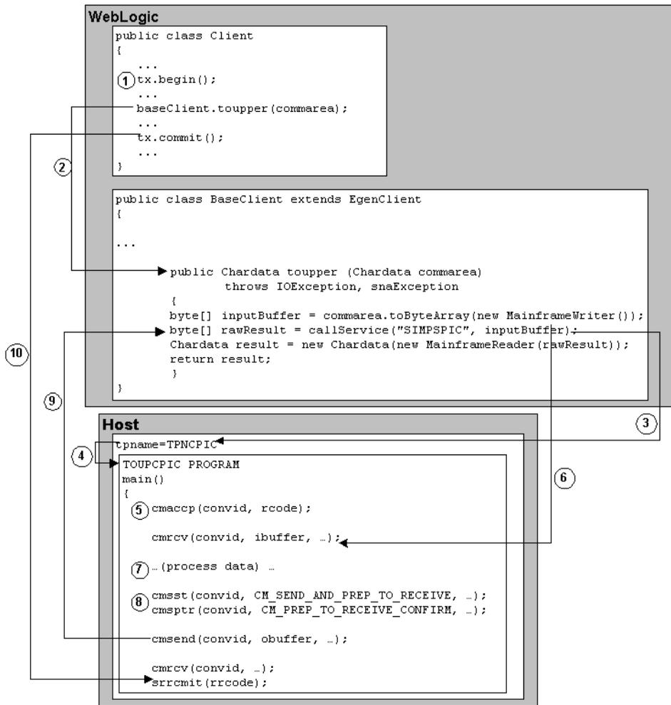
The following steps describe the transactional Java client request/response to a host CPI-C programming flow.
