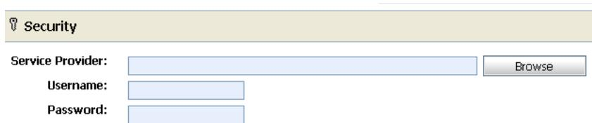
If you specify a proxy service provider in the test console, all client-side PKI key-pair credentials required by WS-Security are retrieved from the proxy service provider. You use the user name and password fields when an operation’s request policy specifies an Identity assertion and user name Token is one of the supported token types. For more information, see [Web Service Policy](#).
