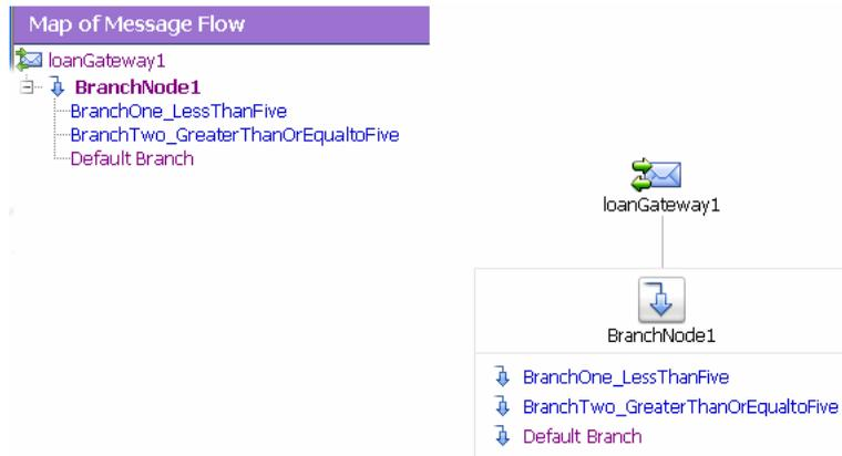
For more information on configuring a conditional branch in a route node, see “Adding Route Node Actions” in [Proxy Services: Message Flow](#) in *Using the AquaLogic Service Bus Console*.
