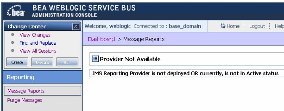
**Note:** In a cluster, the JMS Reporting Provider is targeted to Cluster. Therefore in a cluster, to view and purge messages, you must configure at least one managed server to run with the Administration server. If no managed servers are running, AquaLogic Service Bus Console displays the message shown in the previous figure.
