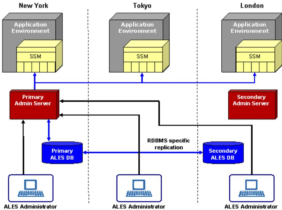
Now consider the case when the data center in New York goes down, illustrated in [Figure 7-3](#). The SSMs detect that the primary Administration Server is down and connect to the secondary Administration Server. The secondary Administration Server detects that the primary database is down and connects to the secondary database server (the replica).
