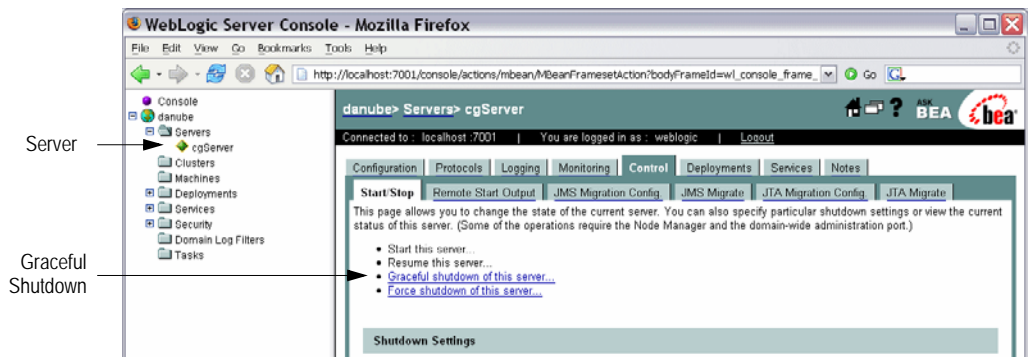
Figure 2-3 Graceful Shutdown of a Server
