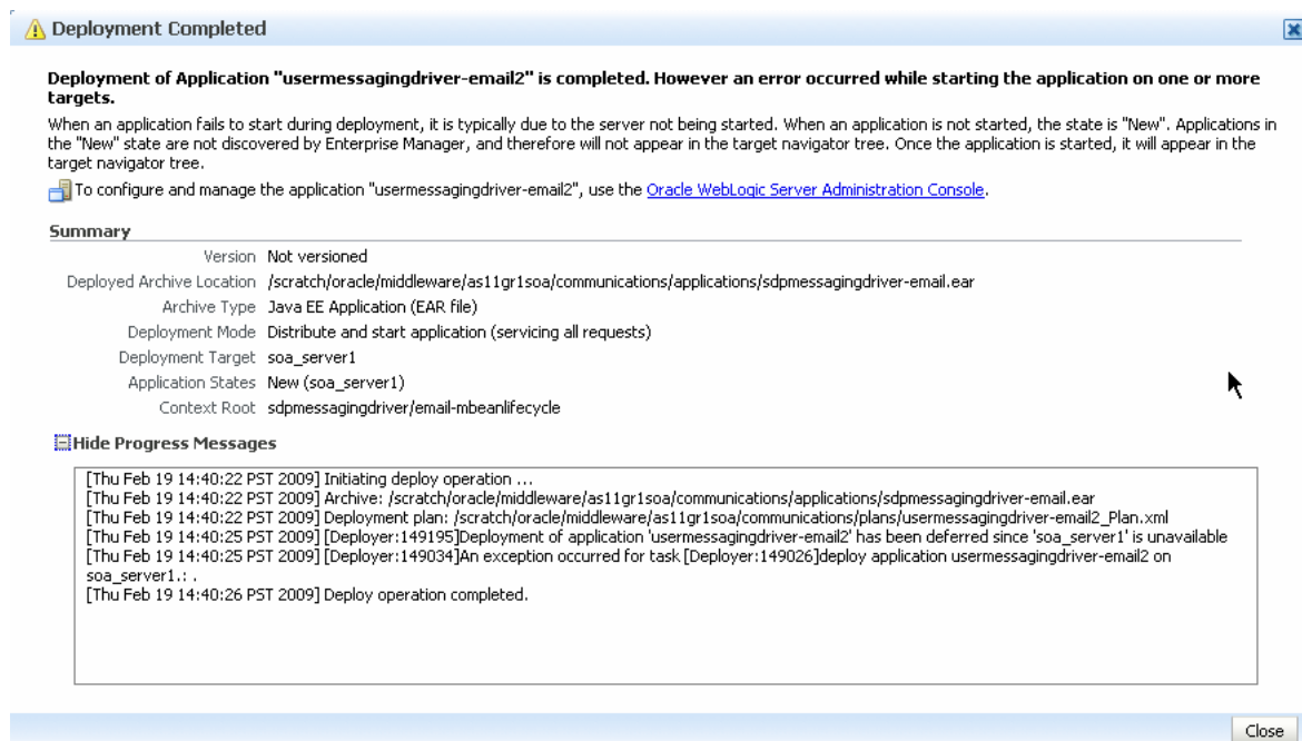
Figure 26–12 Deployment Completed screen
